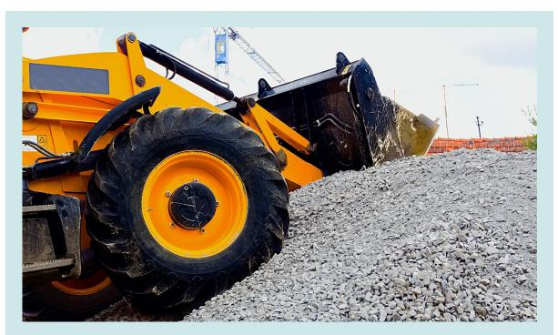
Contractor Ltd replaced the tyres on its front–end loader with solid-fill puncture-proof tyres. These are tyres that have been injected with a liquid that cures to form a soft rubber core. This eliminates flat tyres and blowouts, and the tyre pressure remains constant for the life of the tyres.
